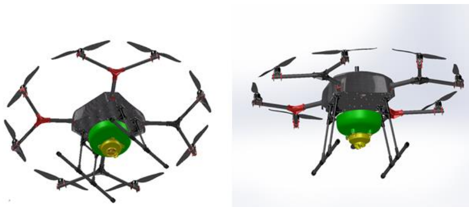
Figure 18: Seedpod releaser attached on CERBERUS UAV.
