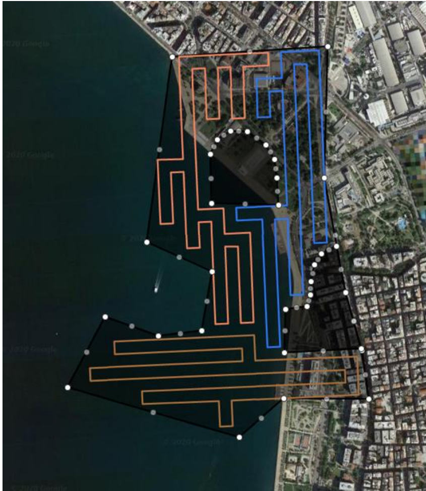
Figure 30 - Concave polygon with multiple obstacles and multiple UAVs
