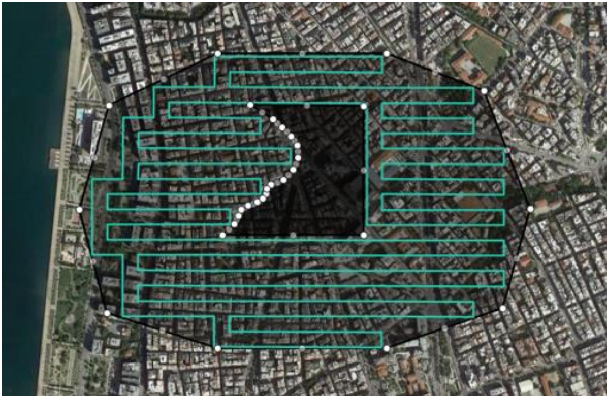
Figure 26 - Path planning of a convex ROI with an obstacle
