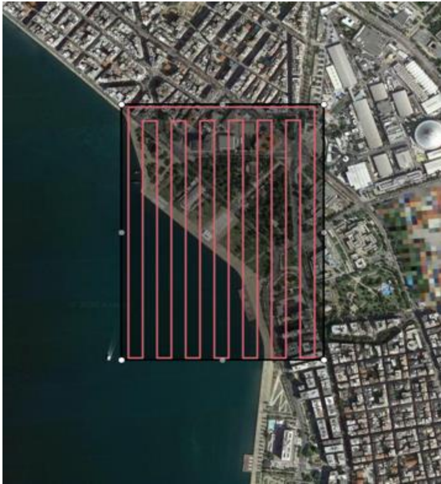
Figure 22 - Path planning of a rectangular area
