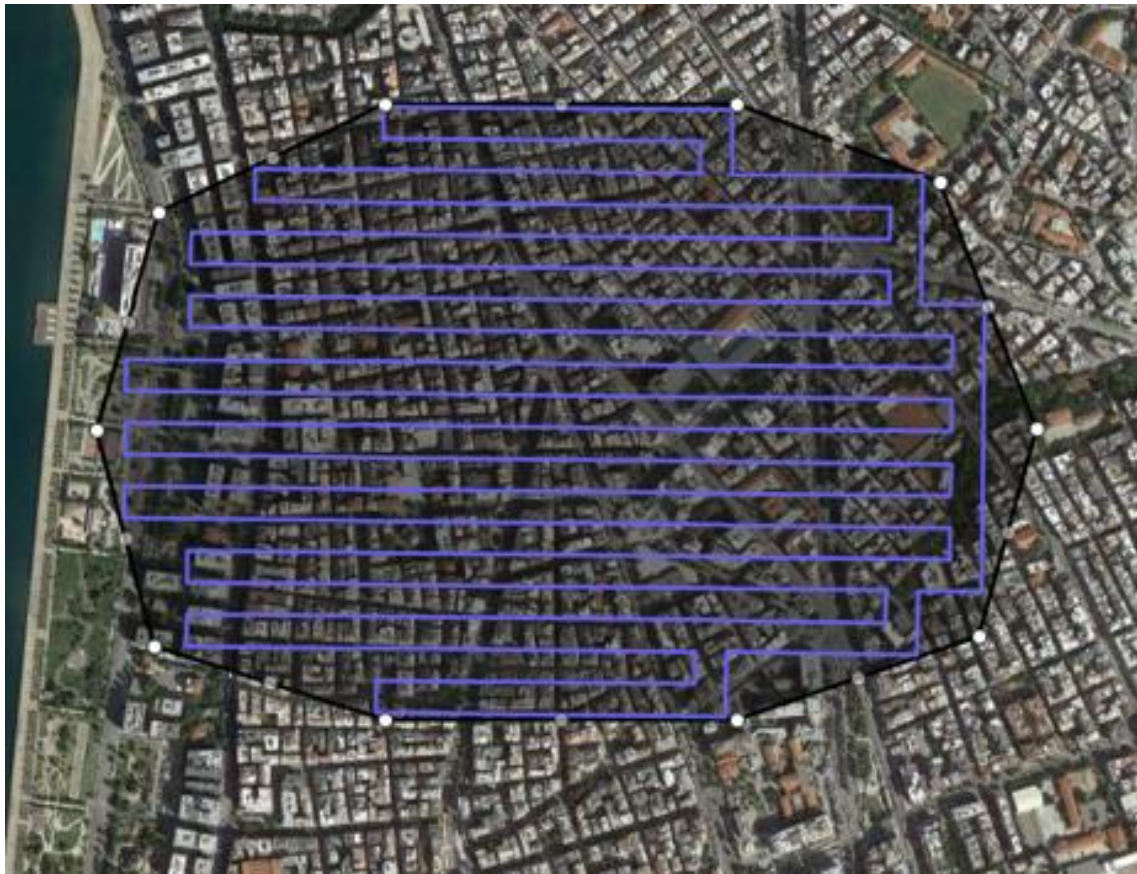
Figure 24 - Path planning of a convex ROI
